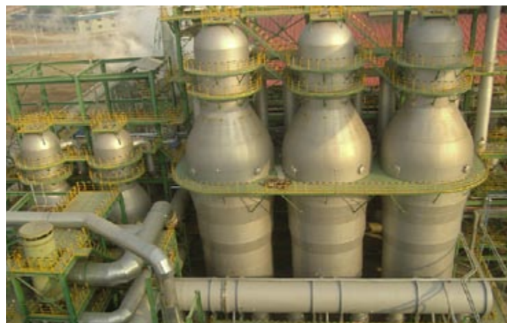
首秦1号高炉热风炉采用的助燃空气高温预热工艺 High-temperature preheating technology of combustion air adopted for hot blast stove for Shouqin 1# blast furnace
