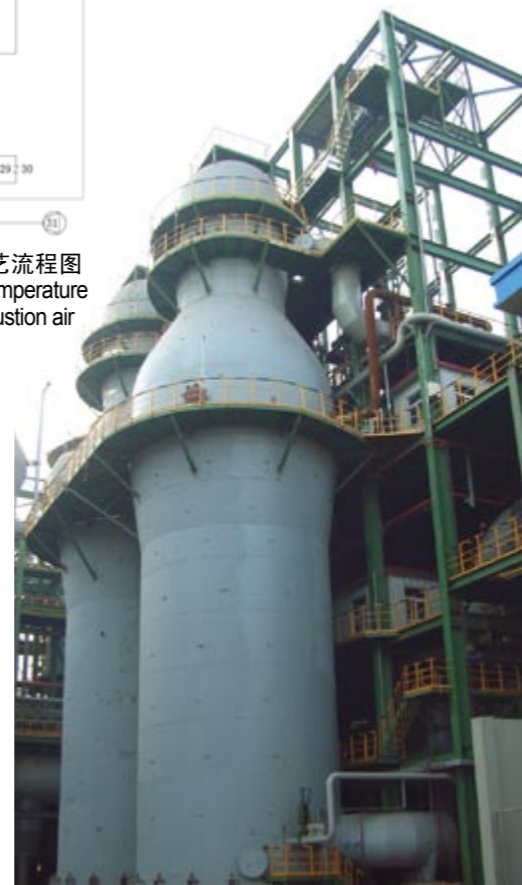
迁钢2号高炉助燃空气高温预热炉 High-temperature preheating furnace of combustion air for Qiangang 2# blast furnace
